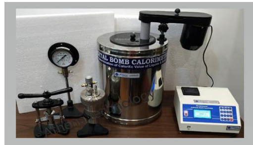
Fig.3. Calorimeter measures the energy content of each coal sample to estimate.
